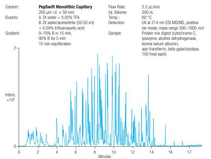
Figure 5: MS chromatogram of a capillary LC separation of over 100 peptide fragments, obtained in less than 15 minutes using a PepSwift column.
