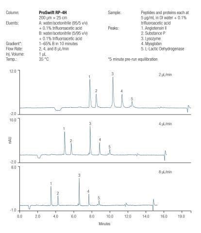
Figure 2: The effect of increased flow rate using the same gradients on the ProSwift RP-4H, 200  $\mu$ m × 25 cm monolith column
