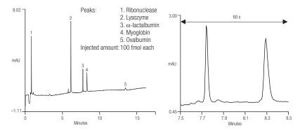
Figure 6: (Left) Separation of 5 proteins using a 200  $\mu$ m ID PepSwift column, and 1. Ribonuclease A (14 kDa), 2. Lysozyme (14.3 kDa), 3.  $\alpha$ -Lactalbumin (25.6 kDa), 4. Myoglobin (17.1 kDa), 5. Ovalbumin (44.3 kDa); and (right) an enlarged region of the chromatogram showing the symmetrical shape and narrow peak widths of peaks 3 and 4
