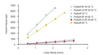
Figure 1: Column backpressure as a function of eluent flow rate at 35 °C and 60 °C for a ProSwift RP-4H, a ProSwift C4 RP-5H column, and a PepSwift column. All column formats are 100  $\mu$ m × 25 cm, eluent: 90.5/9.5 water/acetonitrile + 0.1% trifluoroacetic acid
