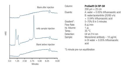
Figure 4: Analysis of a monoclonal antibody on a 200  $\mu$ m x 25 cm ProSwift C4 RP-5H column demonstrating no protein carryover between runs
