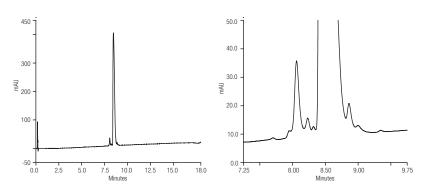
Figure 8: Separation of mAb variants using a 500  $\mu$ m x 10 cm ProSwift C4 RP-5H column. The separation was performed at a temperature of 85 °C and a flow rate of 150  $\mu$ L/min using a gradient from 12–55% B over 15 minutes with 97.5/2.5 (v/v) water/acetonitrile + 0.1% trifluoroacetic acid for eluent A and 10/90 water/acetonitrile + 0.08% trifluoroacetic acid for eluent B.
